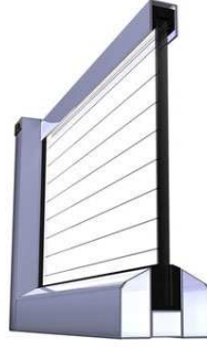
Fig. 48: Single glazing window as reference ( U -value= 5.7 \text{ W/m}^2\text{K} , g -factor= 0.83 ).
